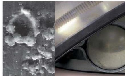
Prevent EDM Pitting and Fluting Damage
