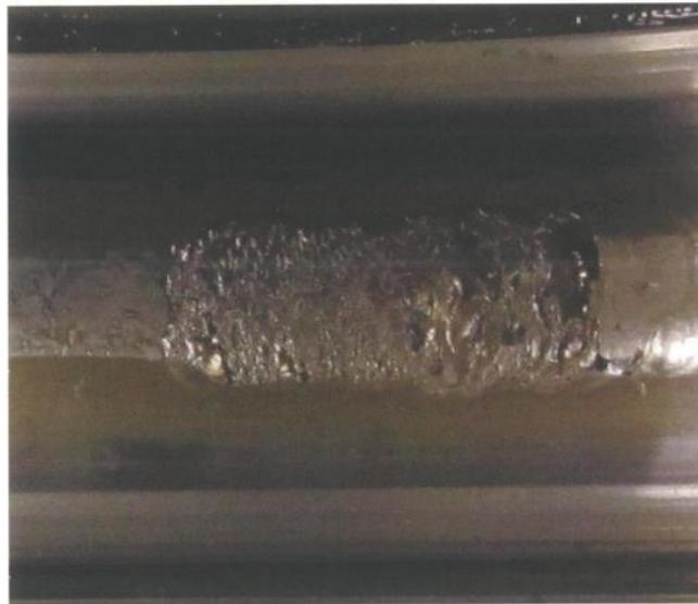
Figure 5: These two photos of the same bearing outer raceway show advanced shaft current / electrically induced bearing damage just prior to failure. Taken September 2011.
